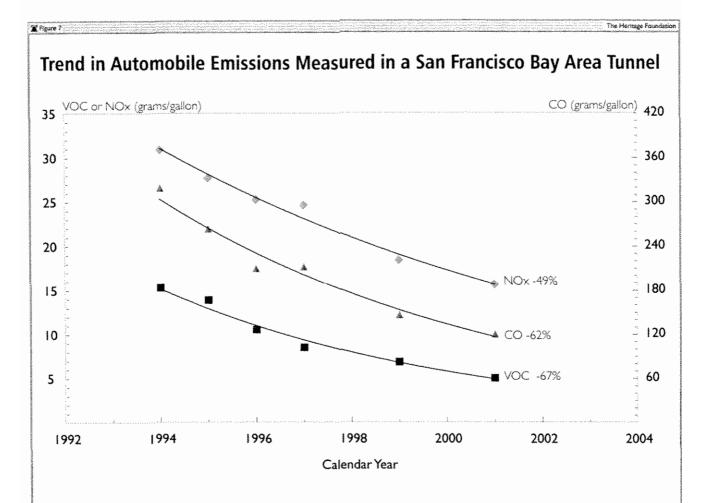
Notes: NOx = nitrogen oxides; VOC = volatile organic compounds; CO = carbon monoxide. Emissions were measured as grams of pollutant emitted per gallon of gasoline burned. Lines through the data points are based on fitting the data to an exponential function.
